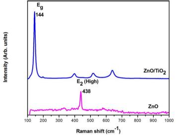
Fig. 3. Raman spectra of ZnO and ZnO/TiO<sub>2</sub> bilayer.
