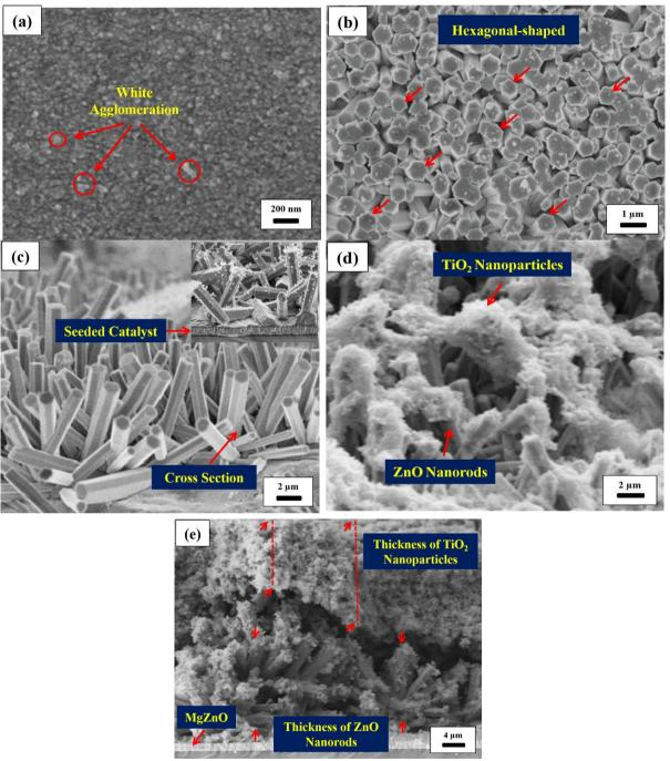
Fig. 1. FESEM images of (a) MgZnO seeded catalyst, (b) top and (c) side view of ZnO nanorods, (d) top and (e) side view of ZnO/TiO<sub>2</sub> bilayer.
